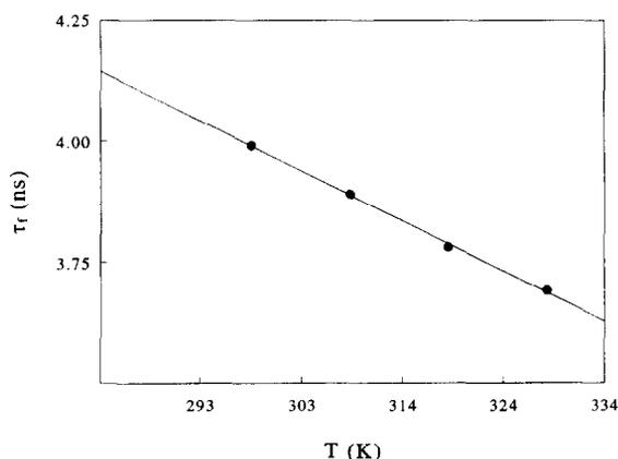
Fig. 4. Plot of fluorescence lifetime( $\tau_f$ ) versus Temperature ( $T$ ) in water.
