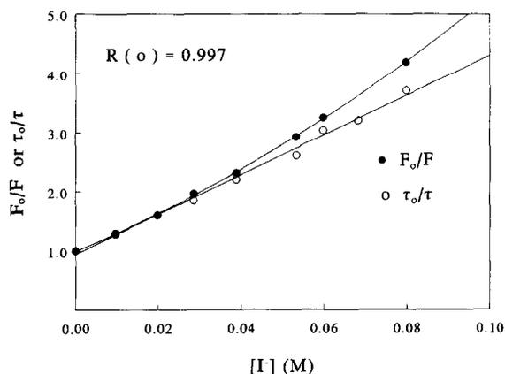
Fig. 7. Stern-Volmer plots for the fluorescence quenching of CAM (pH 5.1) by  $I^-$  ion.
