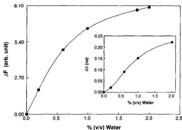
Fig. 5. Plot of fluorescence intensity change ( $\Delta F$ ) and change of lifetime ( $\Delta\tau$ ) (inset) as a function of % (v/v) water in acetonitrile.
