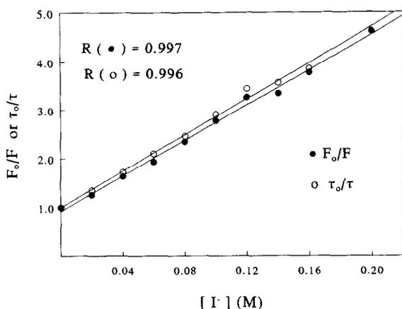
Fig. 8. Stern–Volmer plots for the fluorescence quenching of CAM-Na (pH 9.2) by  $I^-$  ion.
