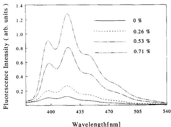
Fig. 3. Fluorescence spectra of CAM in cyclohexane containing various percentage of methanol,  $\lambda_{\text{ex}} = 350$  nm.
