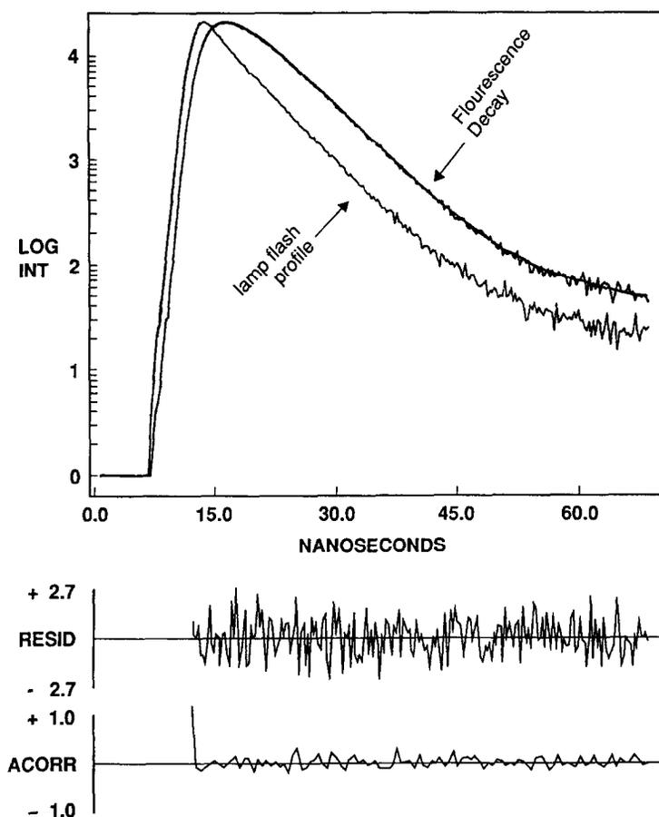
Fig. 2. Fluorescence decay of CAM in acetonitrile solvent,  $\lambda_{\text{ex}} = 337 \text{ nm}$ ,  $\lambda_{\text{em}} = 430 \text{ nm}$ .
